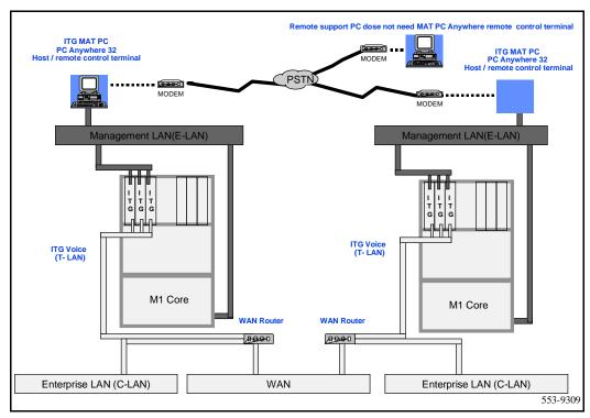
A single network drive location is chosen during the MAT client PC installation process. For multi-system configurations where large data store requirements exceed the capacity of a single drive, or where data integrity is highly valued, a Redundant Array of Inexpensive Disks (RAID) storage solution would be recommended. Tape (or other) backup would be highly recommended.
